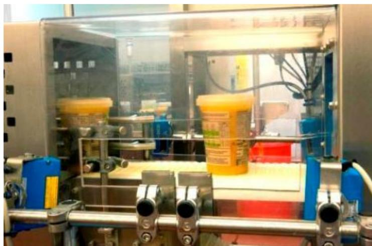
The AutoCoding system sets-up and controls the inkjet printers, whilst an array of barcode scanners check the pots are correct
