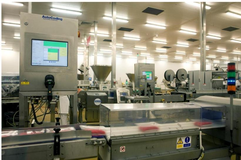
Dedicated line terminals set-up and control the coding and scanning equipment on the packaging lines
