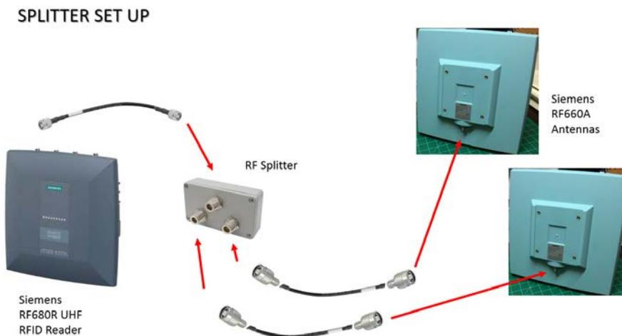
Figure 3: Showing how using an RF Splitter can allow for additional antennas to be added to a port.
