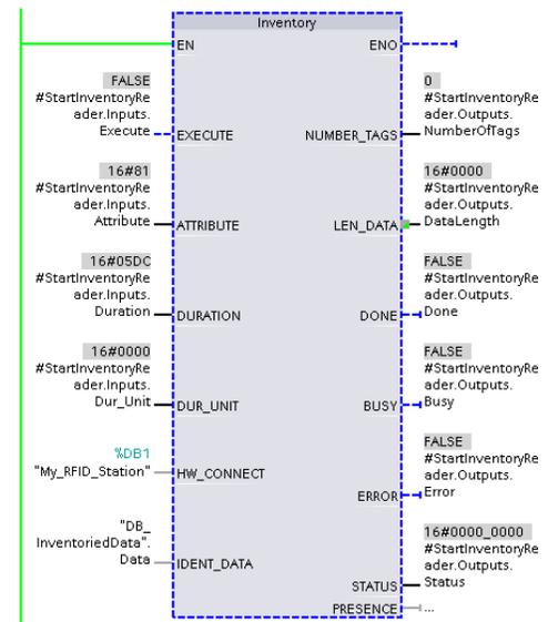
Figure 1: An example of the Inventory block used in a Siemens TIA Portal program. When the Inventory block is executed, the WBM Tag monitor can run at the same time.
