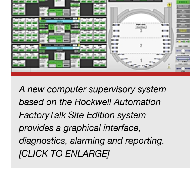
A new computer supervisory system based on the Rockwell Automation FactoryTalk Site Edition system provides a graphical interface, diagnostics, alarming and reporting. [CLICK TO ENLARGE]
