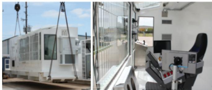
Figure 1: The Infinite Automated Drilling System from DePeuter Electrical Systems uses the SIMATIC S7-400H PLC as its core controller.
