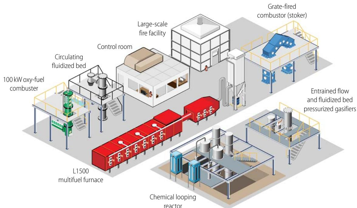
Figure 1: The ICGRF at the University of Utah performs research on coal, shale oil, biofuel, municipal waste, and other fuels for the U.S. Department of Energy, major U.S. utilities, Praxair, and other companies. The entire facility is controlled by Opto 22 automation systems.
