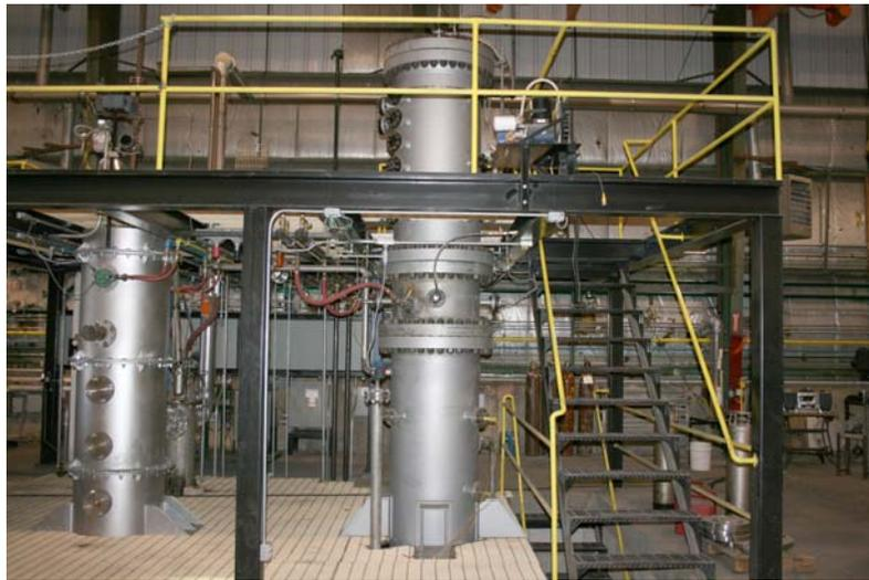
Figure 2: The pressurized fluidized bed gasifier processes solid fuels such as biomass to investigate fuel reactivity, tar production, and quality of synthesis gas.
