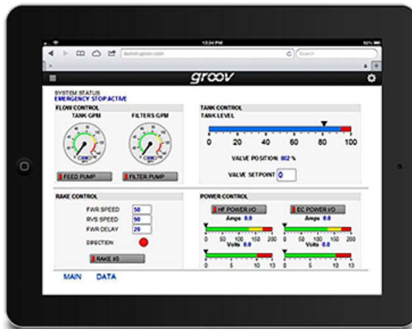
Key parameters for a mobile water treatment system are monitored and controlled using a tablet.
